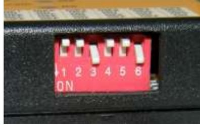
**NOTE:** When moving DIP Switch down, it becomes ON. Please look at the picture above, both DIP3 and DIP6 are in position ON.
