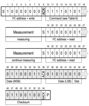
**Figure 16** No Hold master communication sequence – grey blocks are controlled by SHT2x. If measurement is not completed upon "read" command, sensor does not provide ACK on bit 27 (more of these iterations are possible). If bit 45 is changed to NACK followed by Stop condition (P) checksum transmission is omitted.
