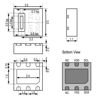
**Figure 1:** Drawing of SHT20 sensor package, dimensions are given in mm (1mm = 0.039inch), tolerances are  $\pm 0.1$ mm. The die pad (center pad) is internally connected to VSS. The NC pads must be left floating. VSS = GND, SDA = DATA. Numbering of E/O pads starts at lower right corner (indicated by notch in die pad) and goes clockwise (compare Table 2).
