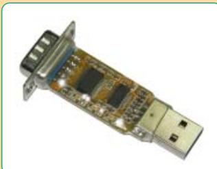
This Board converts Signal from RS232 PORT to mini USB PORT, it is inexpensive. It directly interfaces with Connector USB 2.0 of computer PC.
