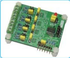
ET-MINI MCP3424 ADC is Board A TO D with 18-BIT 4-CH, run as I2C Interface. Use IC No.MCP3424 of MICROCHIPS to measure both Signal Current and Voltage as SINGLE END MODE (0-2V) and DIFFERENTIAL MODE (+2V, +2V).
